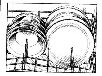
The rack is designed so dishes can be centered behind a single tine and held in place by the rack's support wires. Dishes can also be loaded at an angle to maximize space.
