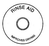
The clear indicator in the center of the cap changes from dark to light when the reservoir is nearly empty. This indicates that it is time to refill the dispenser.
